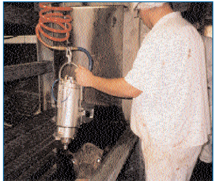
Jarvis' USSS-1 Pneumatic Stunner being used in Australia at Cargill Foods' Wagga Wagga processing plant.
